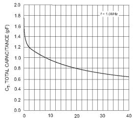
$V_{R^{\prime}}$  REVERSE VOLTAGE (V) Fig. 4 Typical Capacitance vs. Reverse Voltage
